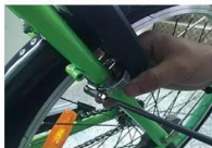
5. Tighten the two screws until the lock is fixed.
