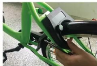
3. Buckle hose clamps on the bicycle rear wheel frame, adjust the appropriate height.
